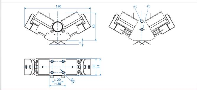
🖲 = Compressed air connection M5 needles extended 🔞 = Compressed air connection M5 needles retracted \* = Stroke
