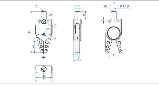
⊕ = Compressed air supply (close) ⊕ = Compressed air supply (open)
