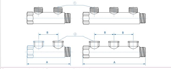
$\bigcirc$  = Connection output (male thread)  $\bigcirc$  = Connection output (female thread)
