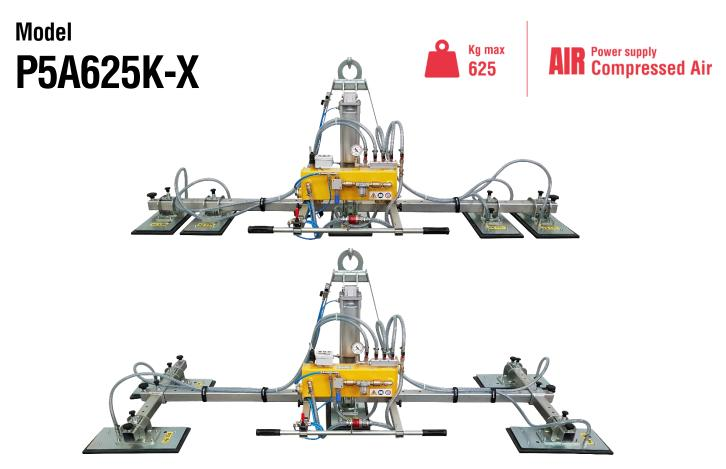
The model P5A625K-X is a **transformable vacuum lifter** with 5 pads and lifting capacity **625 kg**. Thanks to two extension arms (L 830mm), this lifter can change configuration from inline-pads, **suitable for kitchen tops**, to cross-pads, **suitable for big slabs**. The standard central beam is 2400mm long. All the 5 vacuum pads feature **support for quick rotation**.
