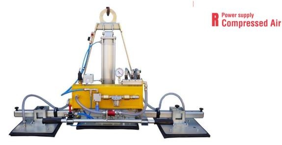
The P3A series of Vacuum Lifters is a range of 3-pads models with lifting capacity **from 375 kg to 2000 kg**. The P3A series is powered by compressed air. The **pneumatic tilting system** allows an assisted movement vertical – horizontal of the load and vice versa. The maximum capacity of the lifter depends on the dimension of the suction plates.
