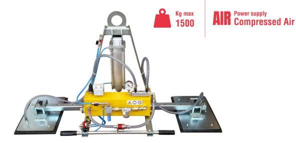
The P2A series of Vacuum Lifters is a range of 2-pads models with lifting capacity **from 500 kg** to **1500 kg**. The P2A series is powered by compressed air. The **pneumatic tilting system** allows an assisted movement vertical – horizontal of the load and vice versa, controlled by a joystick on the lifter's handle. The maximum capacity of the lifter depends on the dimension of the suction plates.
