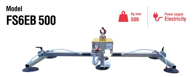
The Vacuum Lifter for sheet metal **FS6 EB 500** is an electric powered model. It is possible to choose between 400V three-phase or 220V single-phase. The pads, equipped with springs, are made of **special oil-resistant vulcanized rubber**, specific for sheet metal.
