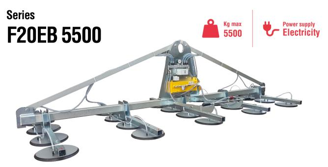
The Vacuum Lifter for sheet metal F20EB is a model with **electric operating system** 400V three-phase or 220V single-phase. The model F20EB 5500 has a maximum capacity of 5500 kg, it has a cross-beam which can be made with different lengths, on standard models L4000 mm, L5000 mm or L6000mm and it has 20 suction pads distributed on 5 arms. The pads, equipped with springs, are specific for sheet metal made in **special oil-resistant vulcanized rubber**.
