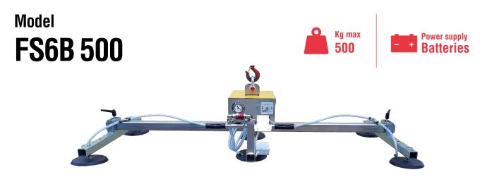
The sheet metal vacuum lifter FS6B is battery powered by high capacity rechargeable batteries (battery charger is included). FS6B has a maximum capacity of 500 kg and **6 suction pads** distributed on 3 cross-arms. The pads, equipped with springs, are made of **special oil-resistant vulcanized rubber**, specific for sheet metal.
