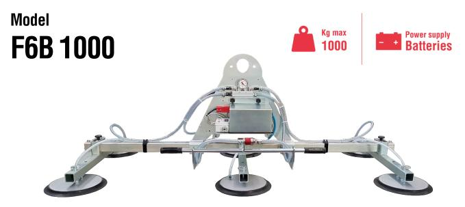
The sheet metal vacuum lifter F6B is battery powered by high capacity rechargeable batteries (battery charger is included). F6B 1000 has a maximum capacity of 1000 kg and **6 suction pads** distributed on 3 cross-arms. The pads, equipped with springs, are made of **special oil-resistant vulcanized rubber**, specific for sheet metal.
