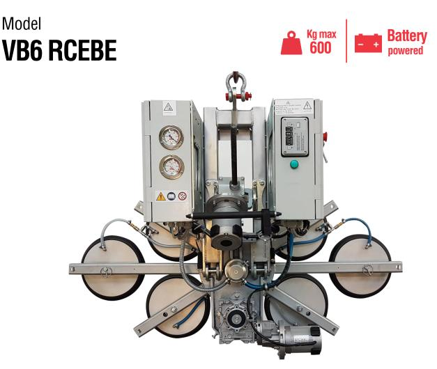
The VB6 RCEBE is a vacuum glass lifter with **electric 360° continuous rotation** and **electric tilting system** 0-90°. It has 6 round pads d. 310mm and the pad spread dimension is mm 1420 x 678.
