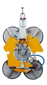
The VB4 d4 is a below-the-hook vacuum lifter suitable for lifting and handling glass units weighing up to 600 kg. Vacuum glass lifter VB4 RCMBM d4 is **battery powered** by rechargeable batteries that, if necessary, may be easily removed and quickly replaced (battery charger included).
