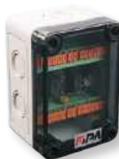
Sensor relay switch box for bundling and logic linking (AND) of sensor signals, since signal inputs on the robot control system are usually limited
