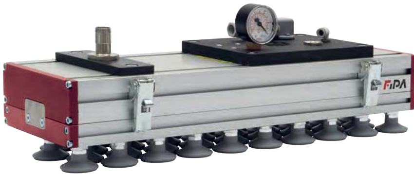
Area gripper SBX-F with vacuum cups diameter 43 mm
