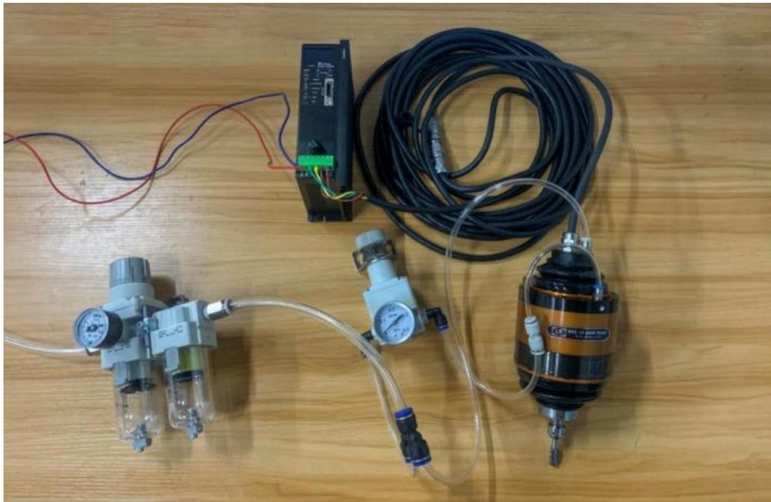
Figure 6-1 Connection of the constant force floating deburring tool system
