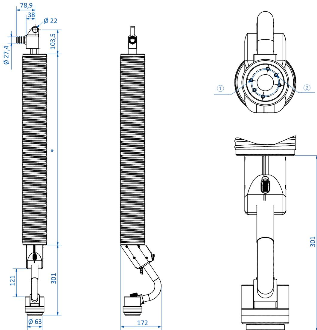
① = Pitch circle diameter 48.5 / hole pattern with 4xM5    ② = Pitch circle diameter 45 / hole pattern with 2xM5
