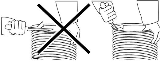
Loosen the protective cover of the operating handle, remove the black tape and unscrew the lifting hose from the plastic adapter. Measure the length of the lifting hose by which it must be shortened to give the FIPALIFT tube lifter the correct height above the ground.
