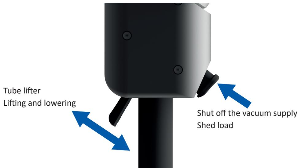
Lifting and lowering: Pulling the „trigger“ operating lever lowers the tube lifter. The trigger is spring-loaded; if it is left unactivated, it returns to its original position and the tube lifter is raised. Actuate the operating lever slowly and carefully, first familiarise yourself with the device without a load.
