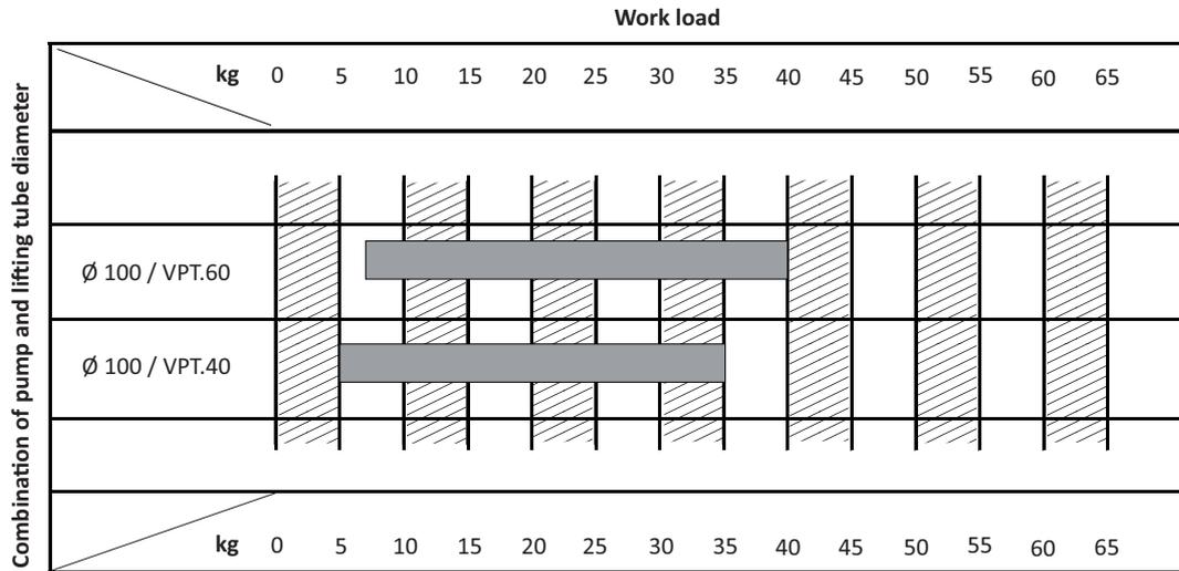
The bars in the diagram show the recommended load weights that can be handled by the respective tube lifter/pump combination. The recommendations are based on appropriate lifting speeds. A light load is lifted faster than a heavy load. A non-porous load, such as a steel sheet, is lifted faster than a porous load, such as cardboard. Do not use the tube lifter/pump combination for heavier loads than those recommended.
