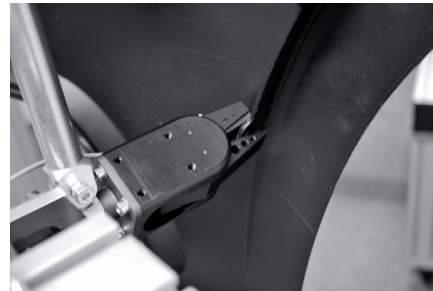
Application example: gripping of plastic flaps
