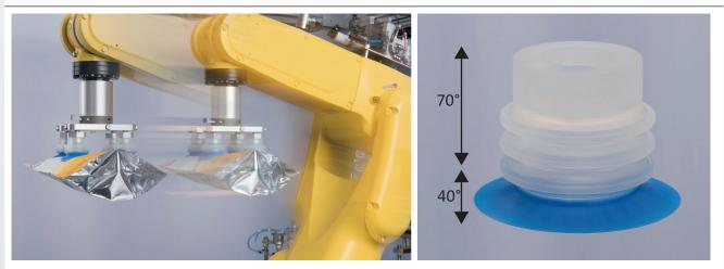
The non-detachable vulcanized, robust bellows area made of silicone 70° Shore A ensures the best possible stability and hold with short cycle times and high acceleration. The soft, conformable sealing lip ensures the best possible seal even on bags with severe wrinkling.
