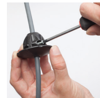
9 Attach the cable retraction stopper to the connector cable about 1 - 1.5 m from the SmartPAD
