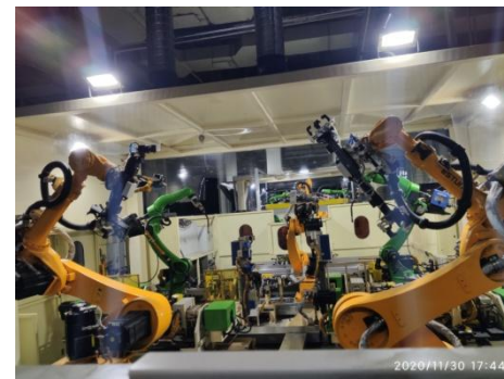
Welding of exhaust pipe of Jinfeng automobile
