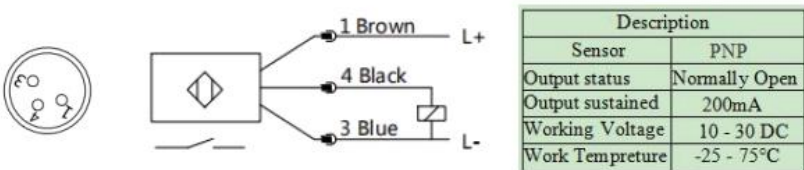
Wire connecting way of Lock/Unlock status sensor
